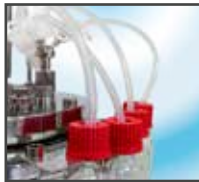
8. Sterile multiple sampling system.
