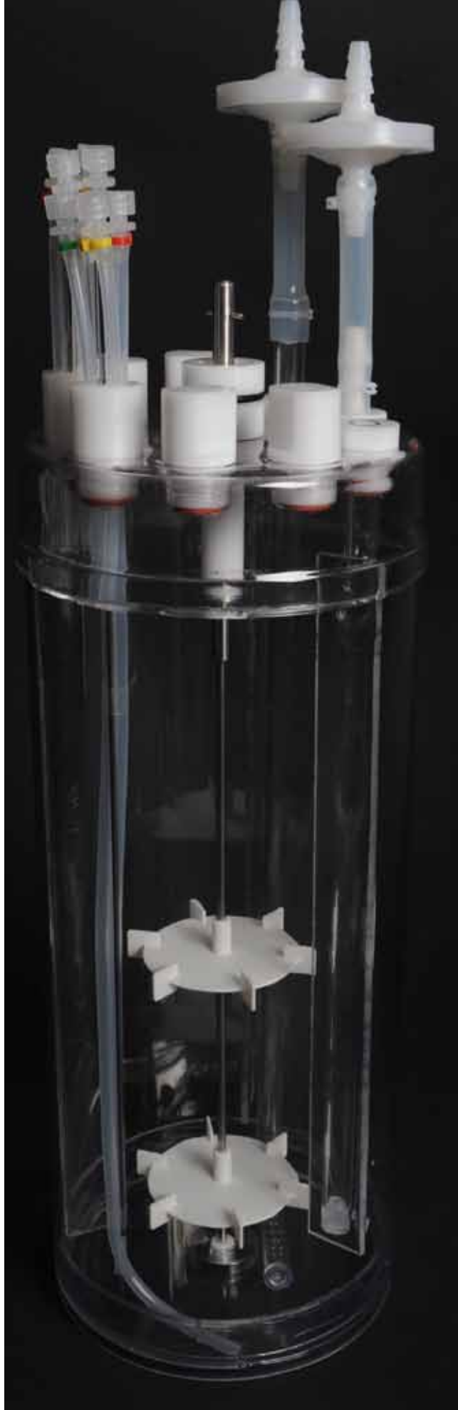
OD130 x 420 mm BactoVessel customised to end-user requirement integrating 3 baffles, ring sparger, dual In&Out, HPD drive and two specific Rushton turbines.
