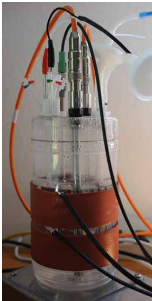
CerCell offer slim line 50x380 mm silicone heating blanket, which fits OD130, 150, 200 mm CellVessel and BactoVessel. Power rated at 110 watt from 48, 110 or 230 VAC supply.
